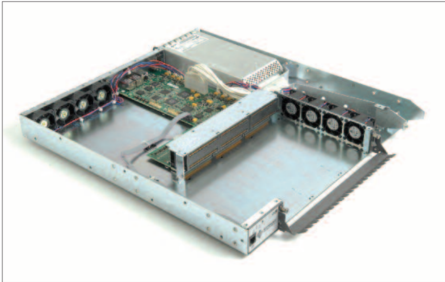
Figure 2. Interior view of MTC5070 with built-in MCH and shelf management, and enterprise class, removable power supply
