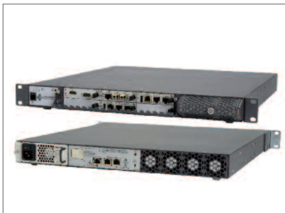
Figure 1. Front and rear view of single rack space MicroTCA platform with front-to-back cooling
